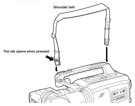
To release the shoulder belt, open the tabs at both ends and disengage.
